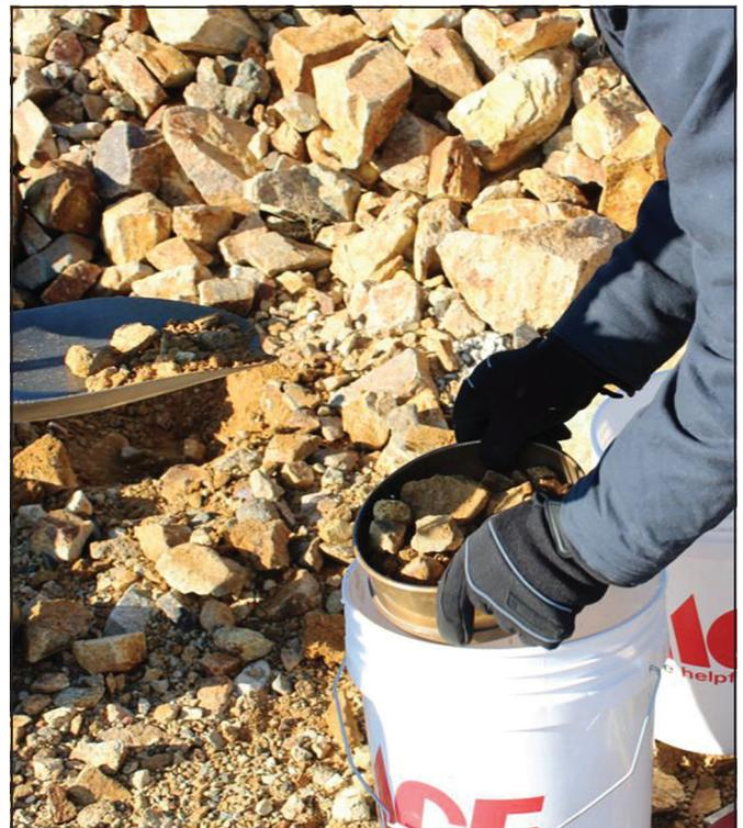
**Figure 5. Sieving mine waste rock pile samples**
