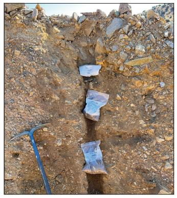
Figure 6. An oxidized profile in a mine waste rock pile, Copper Flat, New Mexico
