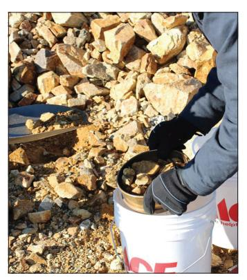
Figure 5. Sieving mine waste rock pile samples
