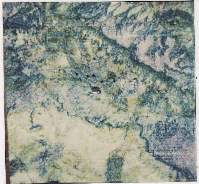
Angle image color composite Ambrosia Lake area. Ratio 4/5 in green, ratio 4/6 in red, ratio 4/7 in blue.
