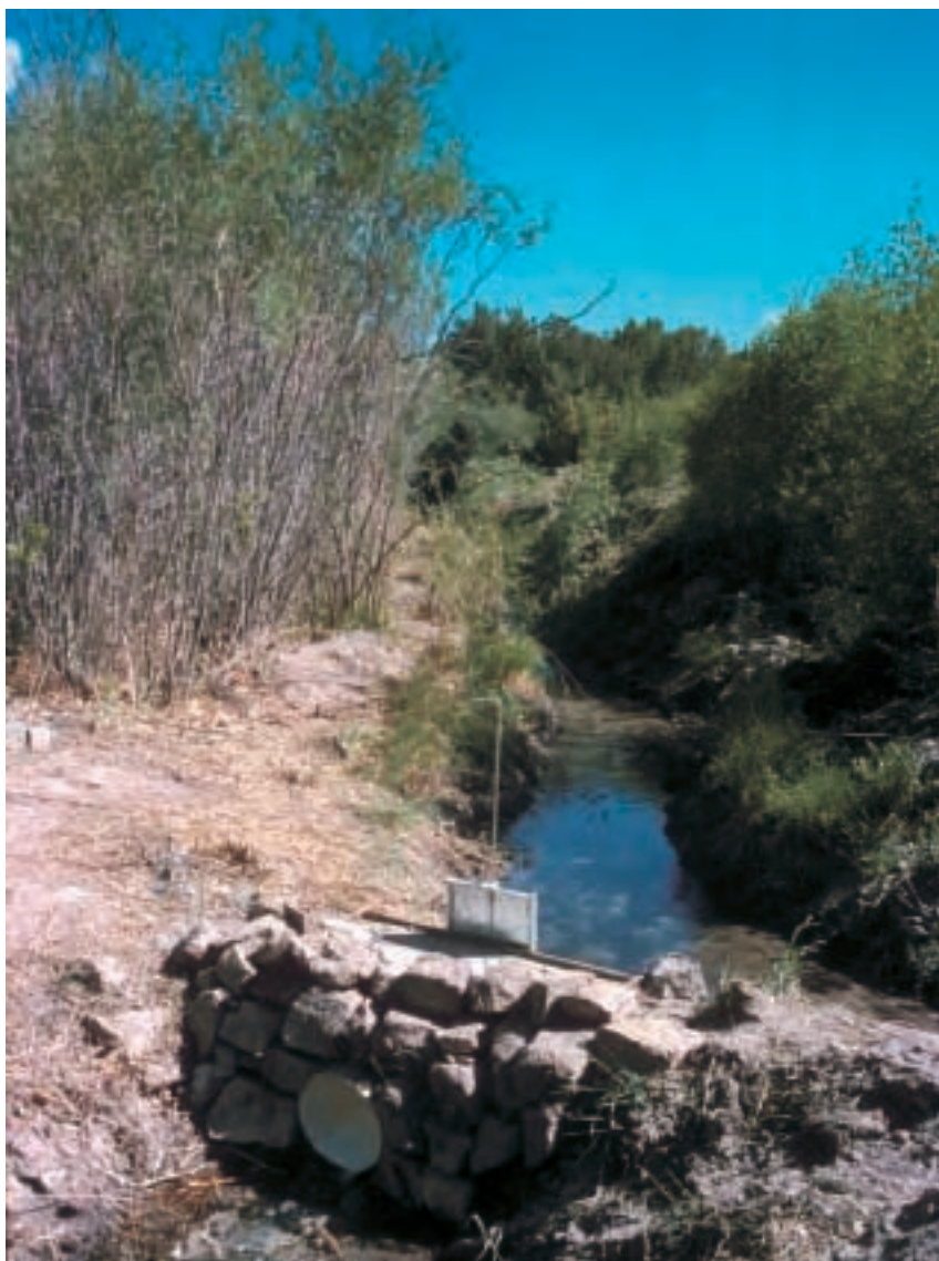
A flume measures discharge from El Oso Spring near the village of Placitas. In Placitas, water rights applications require the Office of the State Engineer to determine whether springs would be affected by the new water use. Photo by Peggy S. Johnson, November 1997.
