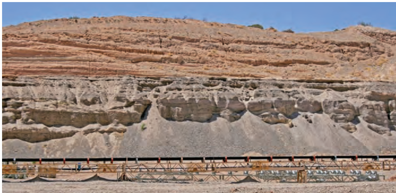
Quarry wall in the Placitas pit, operated by Lafarge North America. The upper reddish overburden layer is unsuitable for aggregate development and must be removed and stockpiled for later use in reclamation. The underlying gray ancestral
