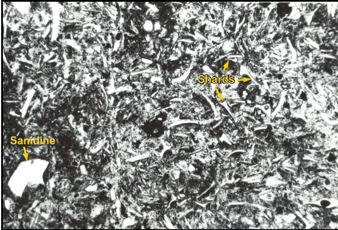
Figure 4. Photomicrograph of vitric tephra from the Abiquiu Formation (Ta) near Cerro Jarosito showing bubble-wall glass shards and sanidine in dusty, glass matrix.
