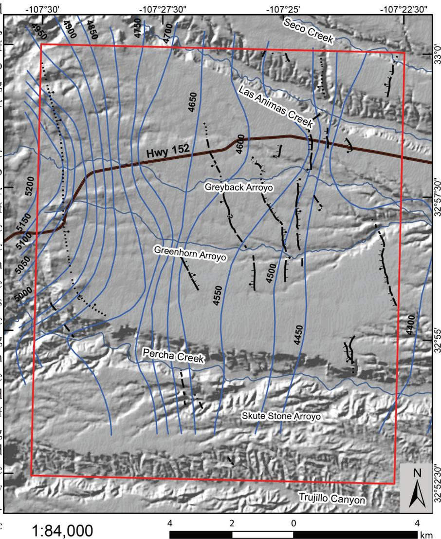
Figure 22—Map showing the potentiometric surface for the Santa Fe Group from groundwater data collected in December-2012 (Jones et al., 2013). Contours are in feet and represent elevation above sea level. Also shown are faults (symbology follows the legend of the Skute Stone Arroyo geologic map). Approximate quadrangle boundary is shown by the red rectangle.
