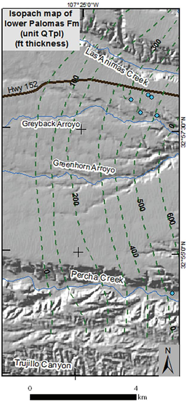
Figure 23—Structural contour map of the base of unit QTpl. Contours are in feet and represent elevation above sea level. Wells used for making the structural contour map are also depicted (blue circles).
