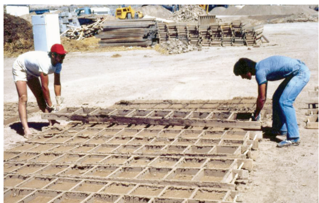
Figure 2. Lifting the ladder mold at a medium-size adobe yard. Photo by George S. Austin.
