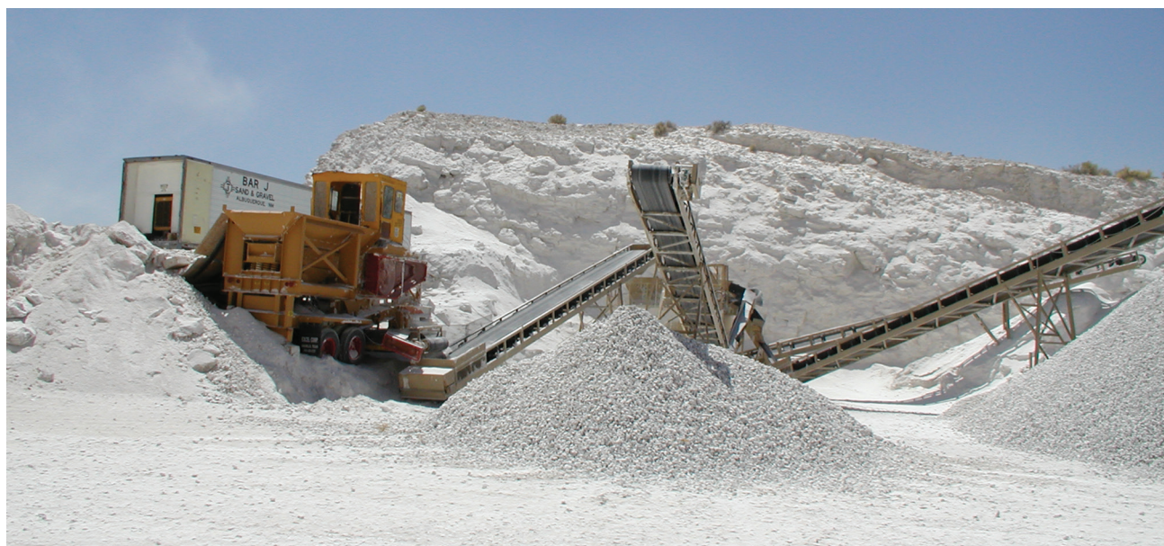
Figure 16. Sizing equipment at the White Mesa gypsum mine (NMSA0170), Sandoval County. Photo by Virginia T. McLemore.
