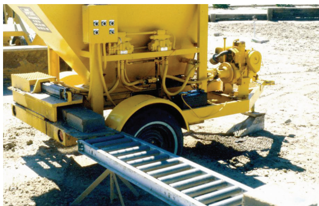
Figure 4. Pressed-earth adobe machine. Photo by George S. Austin.
