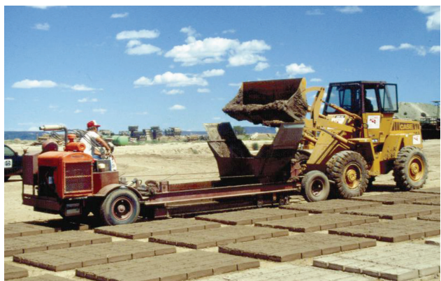
Figure 3. An adobe-laying machine at a large-scale adobe yard. Photo by George S. Austin.
