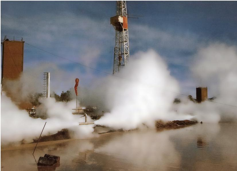
Flow test of HDR (hot dry rock) well back in the early 1990s, EE-2 is brown tower on right, EE-3 is on left. *Photo by Don Brown (LANL, retired).*
