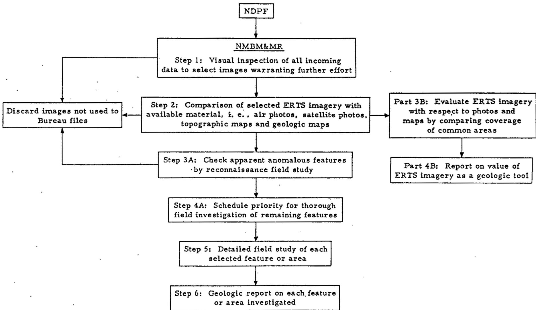
FIGURE 4. Flowsheet illustrating procedure to be followed with each set of images received.
