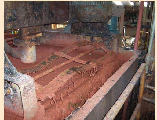
Sylvinite ores from underground mines are crushed and ground in saturated brine. Clay minerals are removed in several stages, and solid-liquid mixture (pulp) is treated with chemicals that render sylvite surfaces hydrophobic (water-repellent). Air is then injected into the pulp and sylvite floats to the surface and is thus separated from halite, which sinks. The froth is then skimmed off with paddles to obtain sylvite concentrate. The red color is from occluded iron oxide minerals in sylvite. Tailings, mostly halite, are stockpiled in tailings dams.
