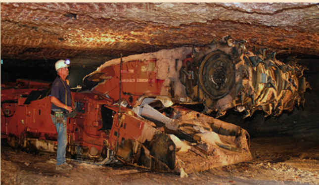
A "continuous miner" at the Intrepid underground potash mine. The drum-like cutter head to the right rotates as it moves into the potash ore. The broken ore drops into the hopper below to be pulled onto a conveyor belt that brings ore to the rear of the miner for hauling to the hoist and plant. The reddish potash in the walls and ceiling show tool marks from the cutter head. Photo courtesy of Jim Lewis of Intrepid Potash.
