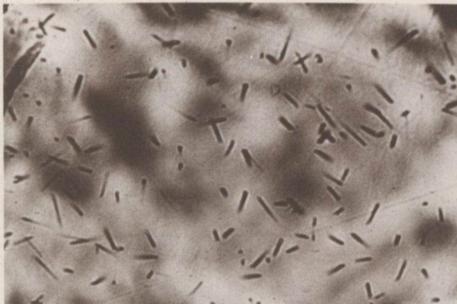
Figure 1—Fission tracks in a crystal of apatite from the large dike that extends south from Shiprock (about 27 million years old). The photograph was taken of a thin slice of the mineral after the tracks had been etched with acid to enlarge them (width of field of view is 0.2 millimeter). Photograph courtesy of Dr. Charles Naeser, U.S. Geological Survey.
