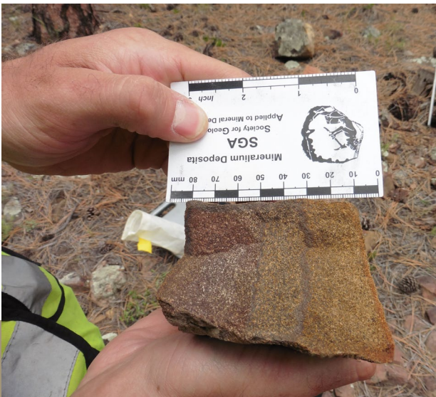
A closeup of a sample from the Apache Mesa heavy-mineral beach-placer sandstone deposit on the Jicarilla Apache Nation. This sample contains 127 ppm total REE and 245 ppm Zr.
