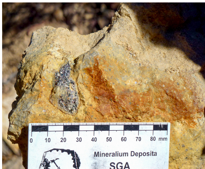
FIGURE 2. Tellurium-bearing pyrite in altered rhyolite, Lone Pine mine. V.T. McLemore photograph, 2013
