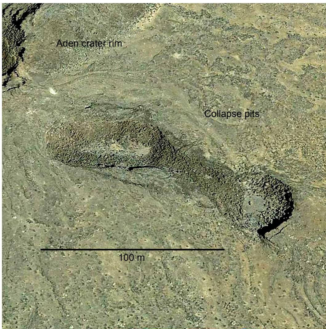
Figure 5. Collapse pits on SE flank of the Aden cone (see Fig. 3), formed by removal of lava from beneath a weak surface crust. The resulting pits are rimless and have blocky interiors.
