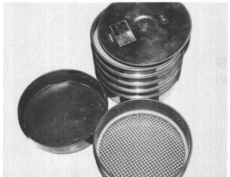
FIGURE 3—Mesh sieves used for determining particle-size distribution.
