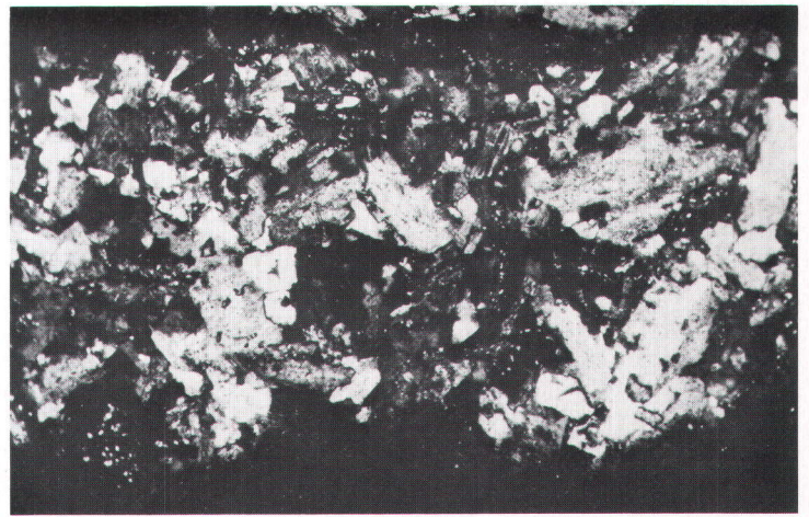
FIGURE 7—Photomicrograph of intrusive rhyolite from 5,700-ft depth in the No. 1 Hurt Ranch well. Plane light; width of field is 1.3 mm.
