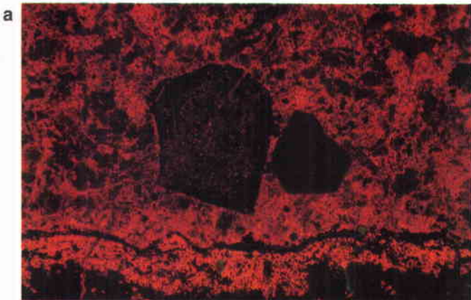
FIGURES 1a & b—1a is a zoned magnetite crystal (red and black) next to smaller apatite (black) in carbonatite (sample LEM CC) under CL. Matrix is carbonate (red). Field of view is approximately
