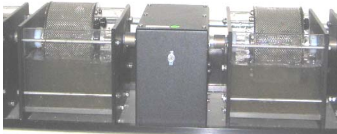
Figure 3. Photograph of the slake durability apparatus consisting of the motor and test drums.
