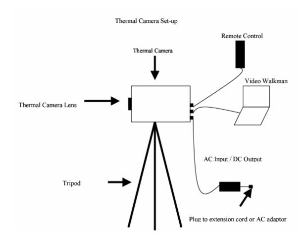
Figure 6. FLIR SC 3000 camera field set-up.
