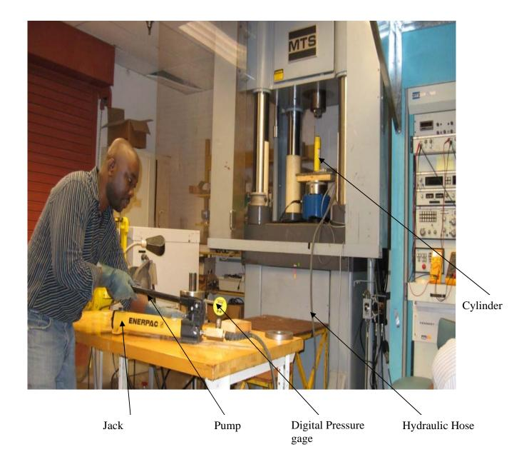
The jacks and hydraulic cylinders which is ENERPAC model are connected by high pressure hoses can carry a maximum oil pressure of 70 MPa or 10,000 psi. A maximum load of 10 tons can be applied considering the hydraulic cylinder cross sectional area of 14.45 centimeters square or 2.24 squared inch. The oil pressure in the hydraulic jacks is indicated by digital pressure gages.
