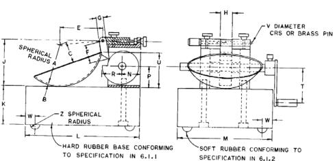
FIG. 1 Hand-Operated Liquid Limit Device
