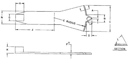
FIG. 3 Grooving Tool (Optional Height-of-Drop Gage Attached)
