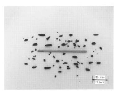
FIG. 8 Lean Clay Soil at the Plastic Limit
