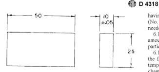
DIMENSIONS IN MILLIMETRES FIG. 4 Height-of-Drop Gage
