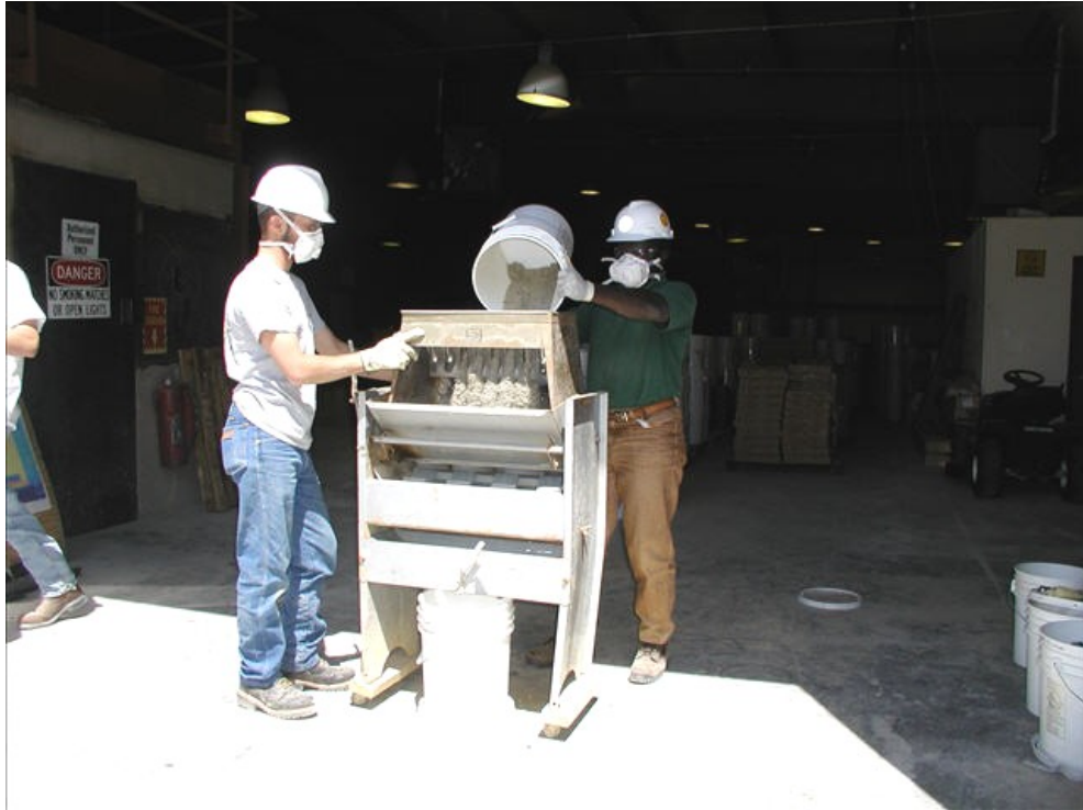
Figure 3.7: Splitting of drill cuttings with a soil splitter.
