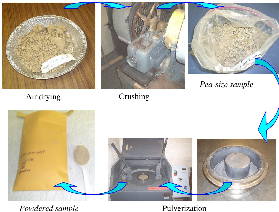
Figure 3.8: Sample preparation processes applied to GHN rock pile samples. The sample is air dried, crushed in a jaw crusher to pea-size, put into a tungsten carbide grinding set and pulverized in a pulverizing machine to get a powdered sample.
