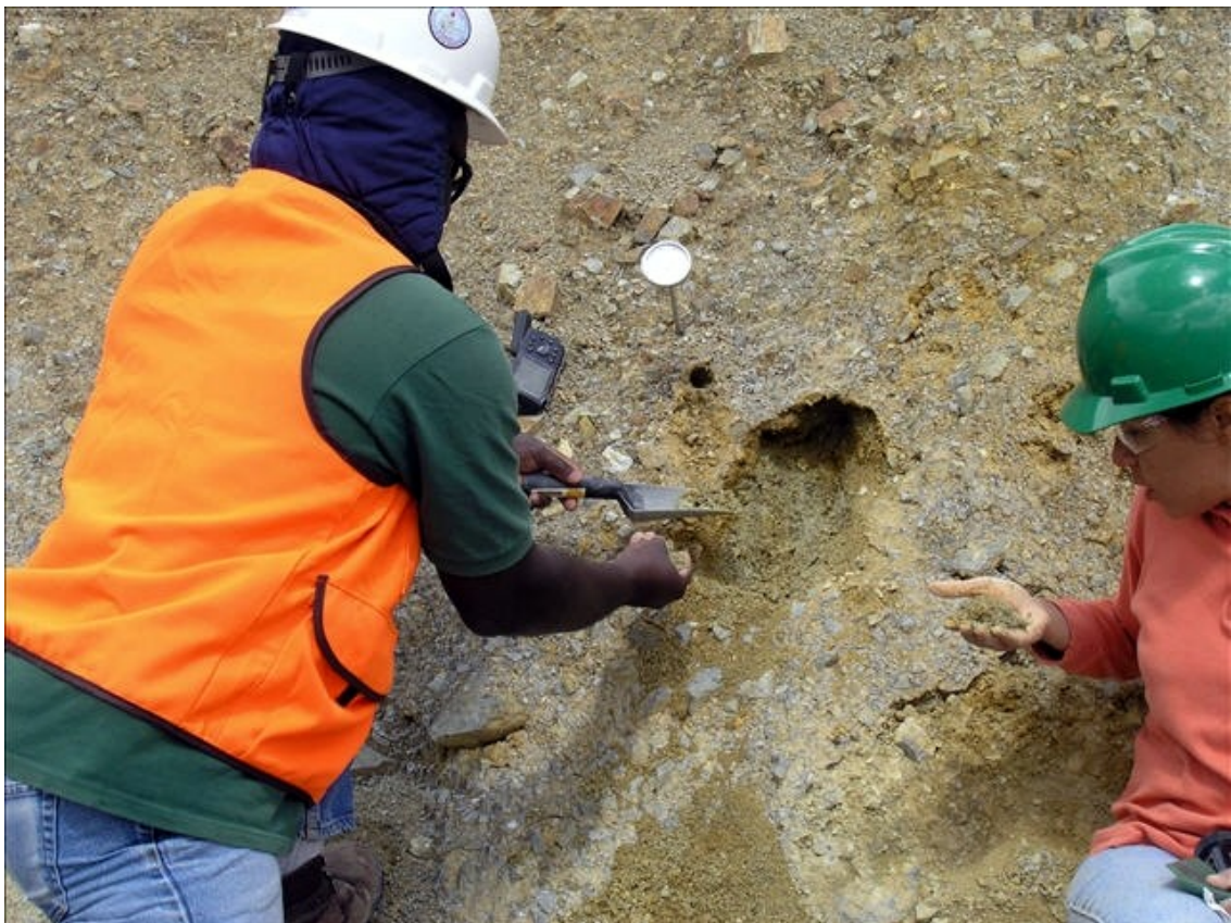
Figure 3.1: Samuel Tachie-Menson and Luiza Gutierrez examining the material for soil properties after collecting a sample. In front of Samuel are a soil temperature probe and a hand-held GPS.
