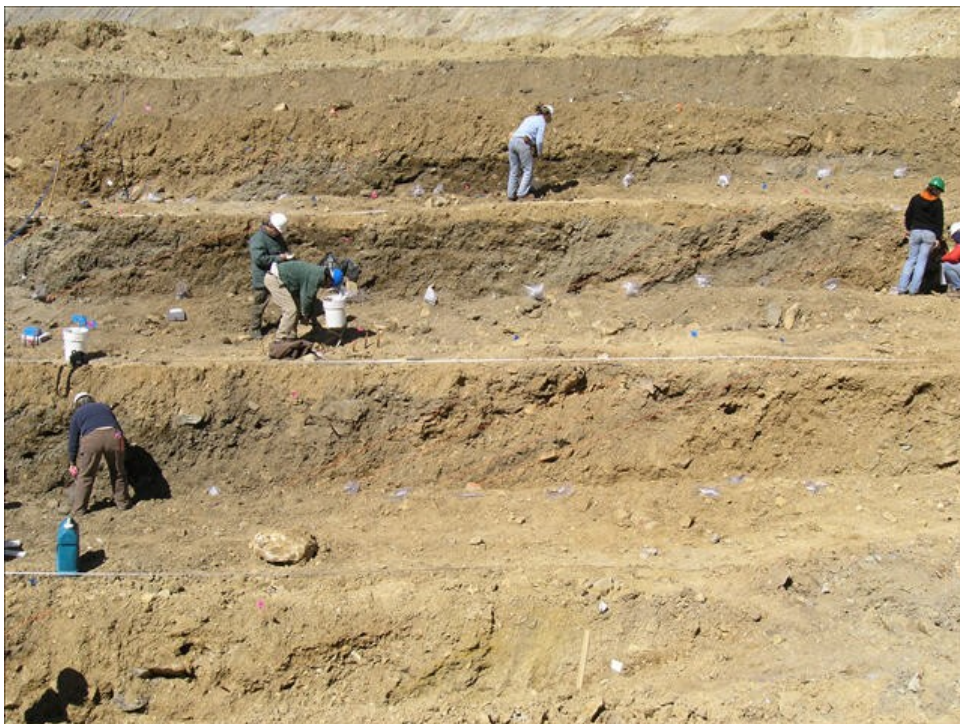
Figure 3.4: A view at the north wall benches of trench LFG-008 as workers take samples. The face of the rock pile is to the left. The little bright objects that are about equally spaced on the ground are Ziploc bags containing samples.
