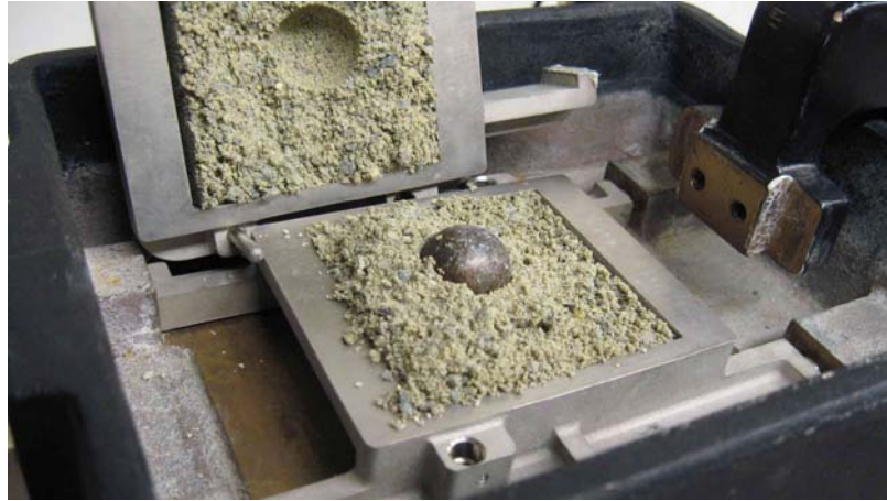
Figure 9: Side view of the shear box containing the steel sphere of 1.90 cm in diameter after completing the shear test.
