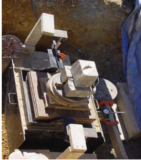
Figure 32: In-situ shear box set up in the field.
