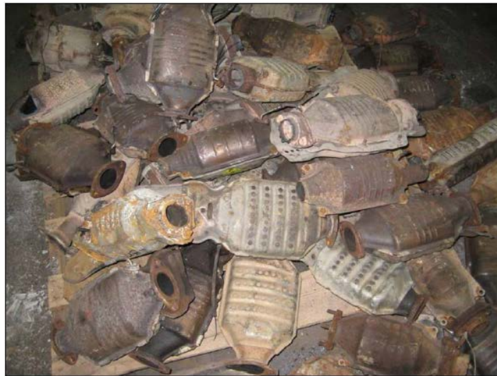
Figure 1. Stockpiled catalytic converters (CATCONs) that have been removed from vehicles before the CATCONs were dismantled and recycled for platinum-group metals. Photograph courtesy of Ashok Kumar, Director, A-1 Specialized Services & Supplies, Inc. Used with permission.
