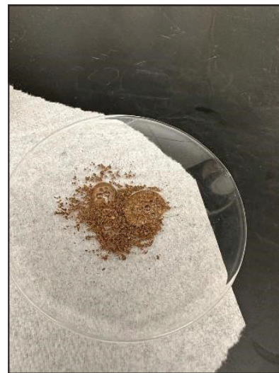
Figure 6. Fizz test on Black Hawk mine waste sample. The photo is illustrating that after adding HCl, sample started to fizz
