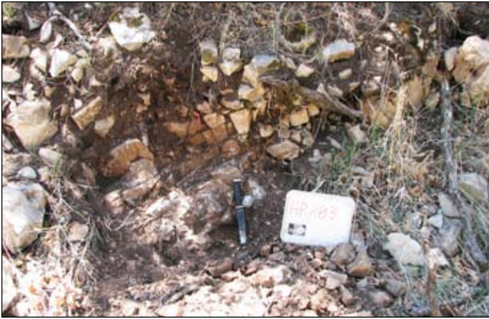
Figure 6 —Thin poorly developed soils that overlay the Yesso Formation. Water must infiltrate through these soils to reach the fractured bedrock below and potentially recharge the groundwater system.
