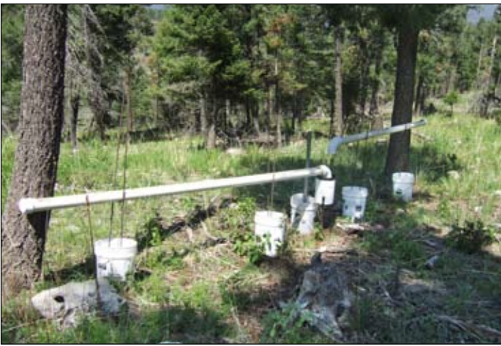
The long troughs catch precipitation under the canopy and guide it into a rain gage.
