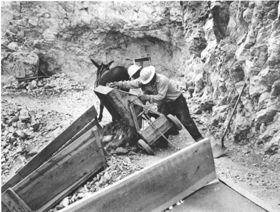
Dumping a small cartload of beryl ore down wooden chute for sorting, 1953. © 1981 Laura Gilpin Collection, Amon Carter Museum, Fort Worth, Texas.
