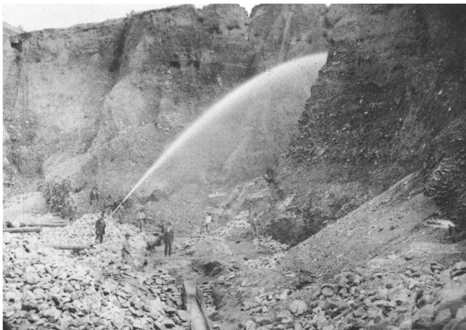
Hydraulic mining on the Lynch placer in either Humbug or Grouse Gulch east of Elizabethtown in the late 1870's. Much of the water used in the placer mines at E'town was delivered by The Big Ditch, a 41-mile-long transmountain aqueduct that originated near the headwaters of the Red River. In hydraulic mining, a firehose-like nozzle, called a monitor, delivers a high-pressure stream of water that washes gravel (and gold) into wooden sluice boxes (visible in the lower center of the photo). Photo by F. C. Warnky, courtesy of the Museum of New Mexico, negative no. 14860.
