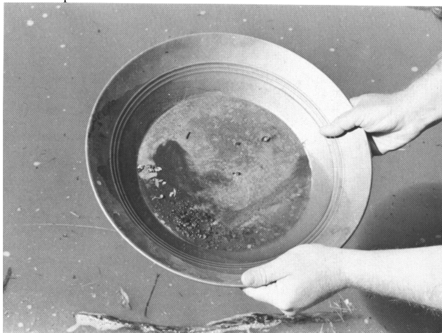
Heavier, dark minerals remaining in the gold pan after washing out most of the light-colored sand include magnetite, garnets, staurolites, and possibly a little gold.
