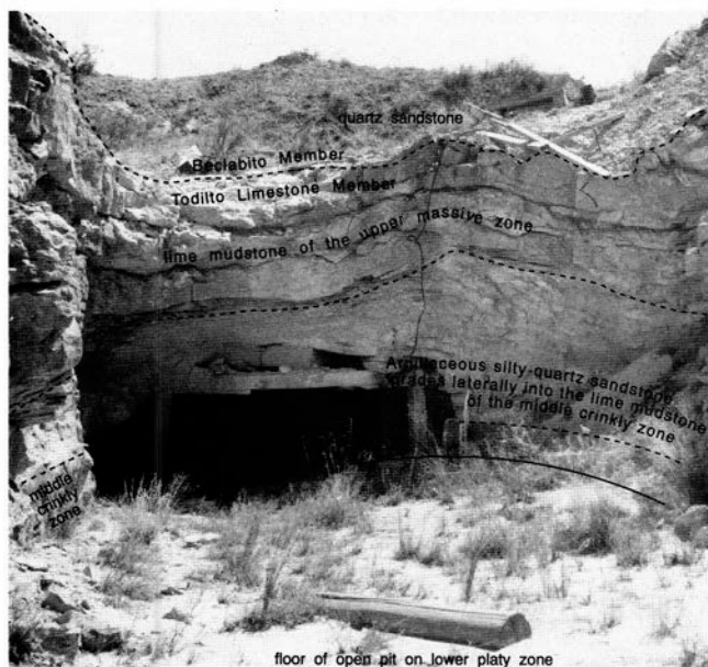
FIGURE 36—View to the south of open-pit and tunnel workings at Section Four, Bunny mine (SE¼ sec. 4, T12N, R9W). The open-pit workings follow the axis and flanks of the intraformational fold, which is developed in the middle crinkly zone. This is overlain by a quartz-sandstone bed within the Todilto Limestone Member that grades laterally into lime mudstones of the middle crinkly zone. The upper massive zone is variable in thickness and contains many solution joints and cavities. The tunnel is some 131 ft (40 m) south of the large portal shown in Figure 35.
