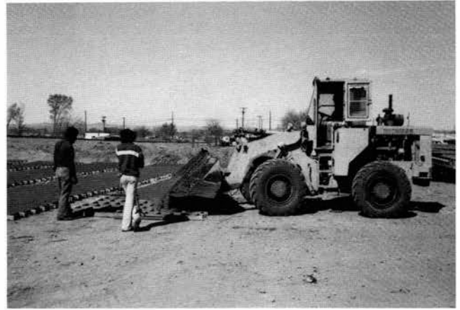
FIGURE 2—Commercial adobe production at New Mexico Earth, Alcade, New Mexico. The front-end loader delivers the semistabilized mud mixture to wooden 10 mold ladder forms. After a few hours, the forms can be removed, leaving the adobes to dry for two to three days, after which they are trimmed and turned on the side to dry for another 10 days to two weeks.
