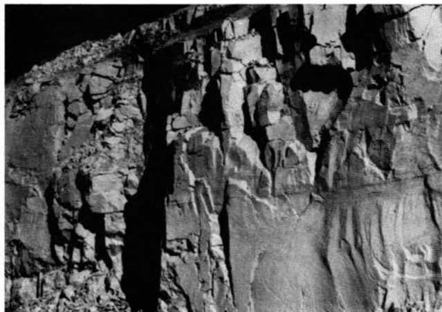
FIGURE 11—Zeolitized tuff exposed in St. Cloud mine. Note laminar bedding and homogeneous, conchoidal fracturing of tuff. Bench height is about 25 ft.
