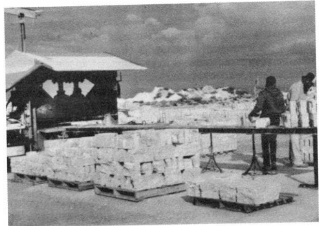
FIGURE 16—Workmen breaking sawed blocks unsuitable for slabbing into split-face ashlar, which is placed on pallets for shipment to customers.
