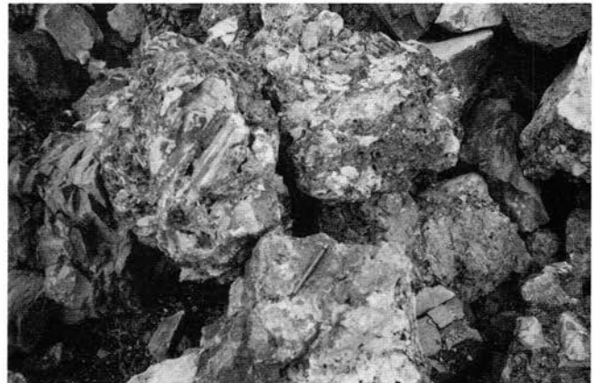
FIGURE 4—Closeup of welded breccia at the Peabody mine aggregate pit. Large pieces of baked shale and siltstone are welded together by glass-like material.
