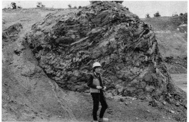
FIGURE 5—Large chimney structure at Peabody mine aggregate pit. The chimney walls consist of welded breccia formed during the venting of combustible gases. All the other material around this structure has been mined out, but this material is firmly in place and cannot be moved.
