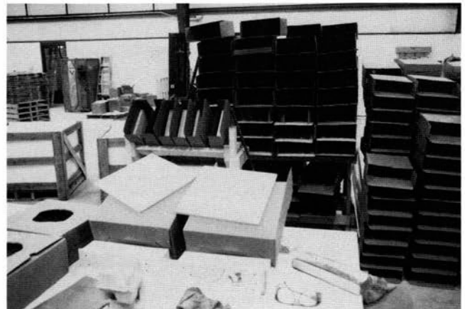
FIGURE 19—Square tiles are packaged, at the end of the tile line, for shipment to customers.
