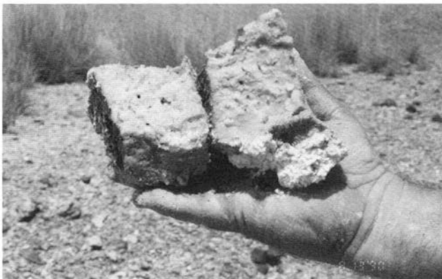
FIGURE 4—Hand specimens of saponite from the north deposit. White magnesite is present at the bottom of both samples.
