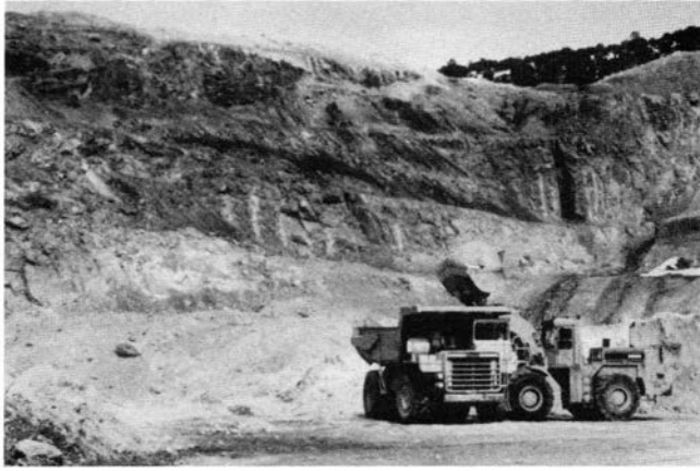
FIGURE 4—Truck being loaded by front-end loader at the Harborlite open pit, No Agua Peaks. The highwall behind vehicles marks local pit margin related to high overburden ratios.
