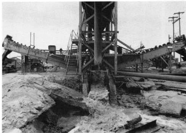
FIGURE 2—Sand plant showing sand screw. Running water concentrates fine-grained heavy minerals.
