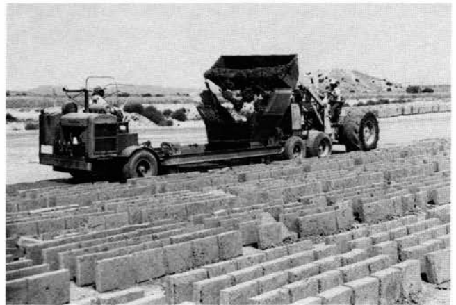
FIGURE 3—Mechanical adobe layer that produces 25 standard-size adobe bricks per laydown. Medina's Adobe Factory adobe yard, Alcade, New Mexico.
