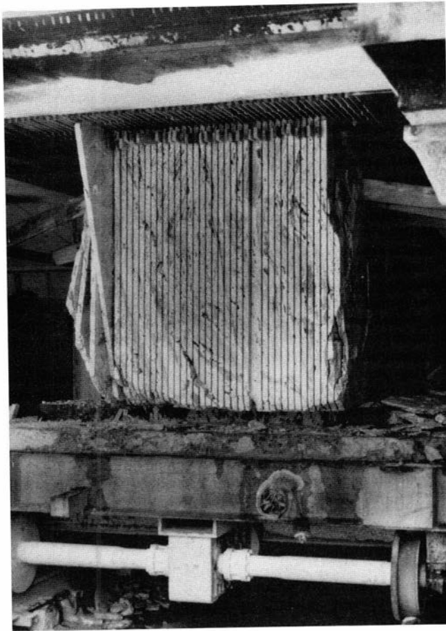
FIGURE 14—Adjustable Gaspari gang saw used to cut stone blocks into slabs. The block was about 4 ft wide before it was slabbed.
