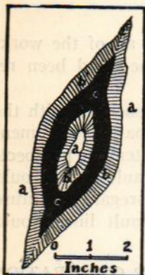
Figure 15.—Sketch of a replacement fragment from the Esperanza claim near Derry. Limestone (a) was replaced by quartz (b) which was followed by fluorite (c).
