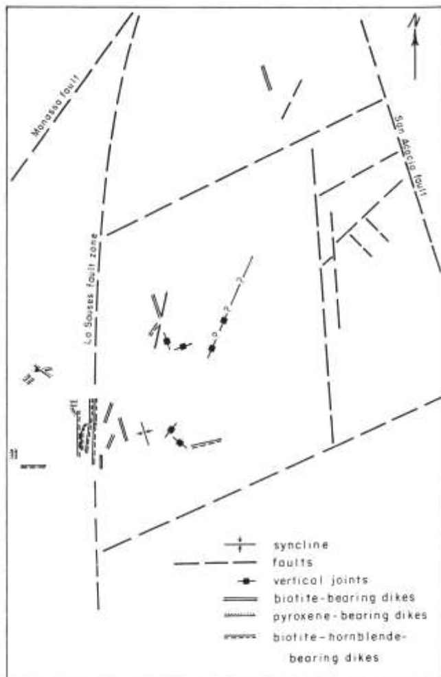
FIGURE N21—GENERALIZED LOCATION AND ORIENTATION MAP FOR THE FRACTURE SYSTEM OF THE SAN LUIS HILLS.
