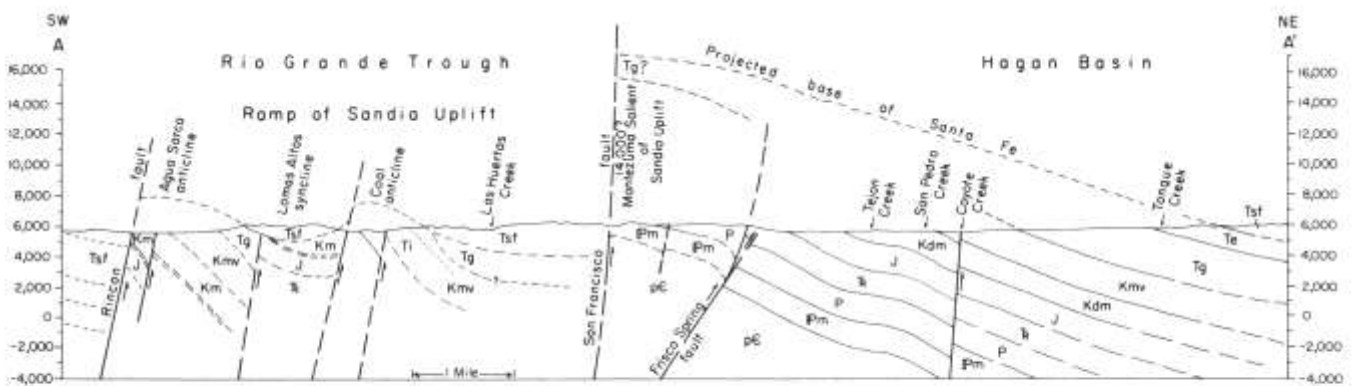
FIGURE S70—STRUCTURE SECTION FROM RIO GRANDE TROUGH TO HAGAN BASIN. Section extends east from Stop S18 area and crosses Montezuma salient and the structural downramp north of Placitas (from Kelley and Northrop, 1975, fig. 63, AA').
