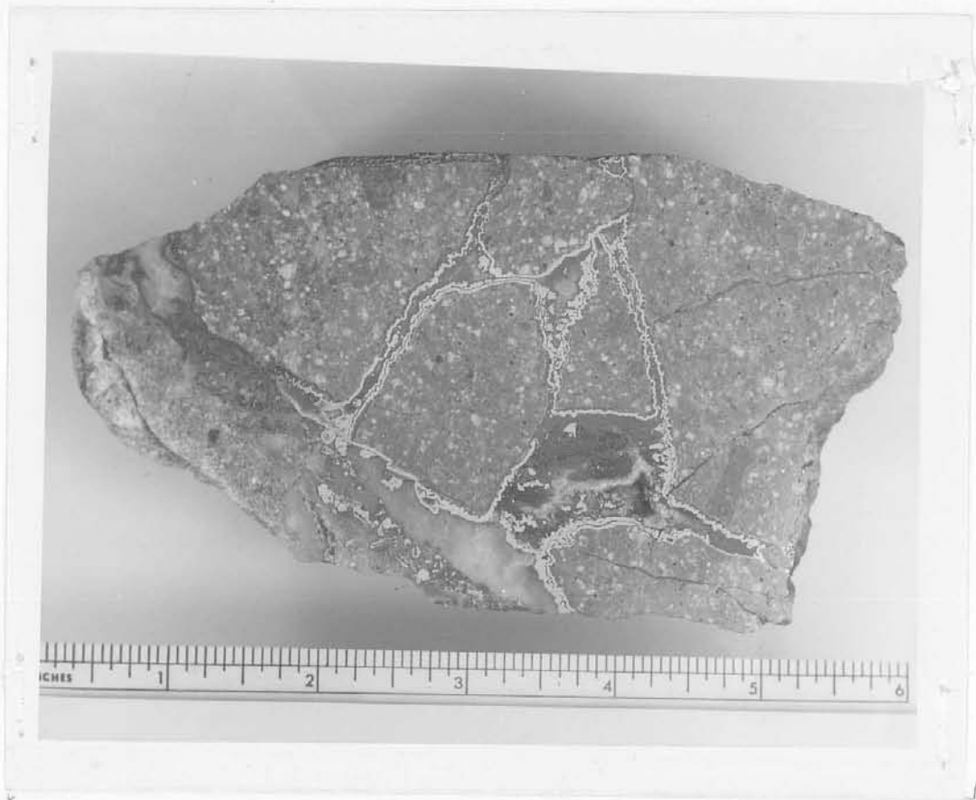
Fig. 13: Polished specimen of the breccia ore from the MCA mine. Bright metallic layers around breccia fragment are manganese oxide; larger open spaces are filled with calcite.
