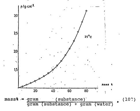
example: Formation of a polytungstate solution with a density of 2.5 g/cm<sup>3</sup>.
