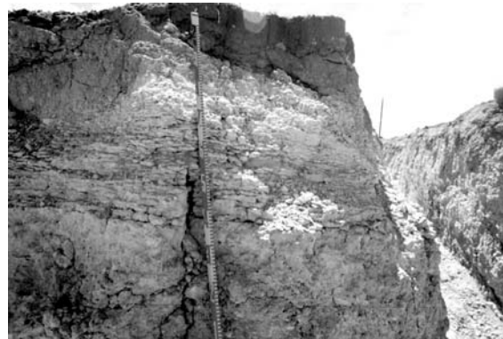
Figure 2-7. Exposure of a petrocalcic soil developed on the Llano de Albuquerque at the Soil Amendment Facility (City of Albuquerque). This exposure is at the east end of a trench cut across an antithetic fault to the San Ysidro (or Calabacillas) fault zone, which was excavated by Jim McCalpin of GEOHAZ, Inc.
