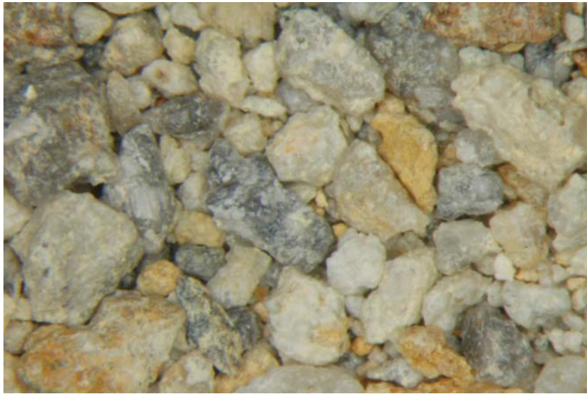
FIGURE A9-62. Photograph of rinsed hand sample showing various rock lithologies. Field of view is 3.5 cm.
