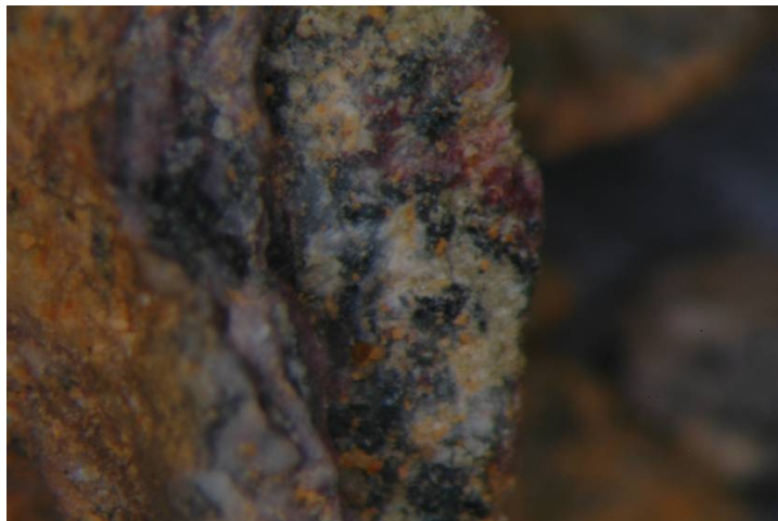
FIGURE A9-55. GHN-KMD-0088. Iron oxides coating rock fragments (field of view is 4 mm).
