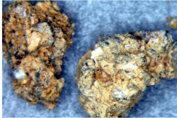
FIGURE A9-27. Figure shows a well cemented rock fragments with Fe-oxide staining. Field of view is 2 cm.
