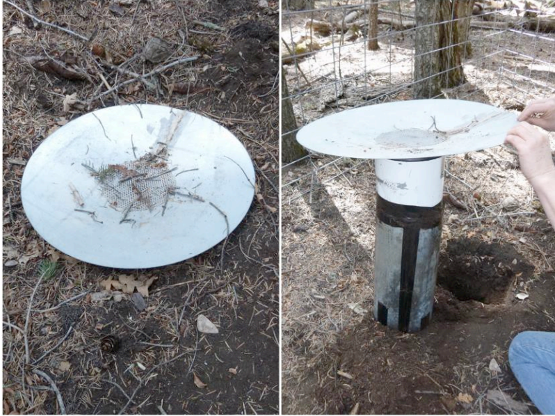
Figure G5: Installation of snow melt collectors. A tipping bucket rain gauge is modified and buried. The collection funnel is on the ground.
