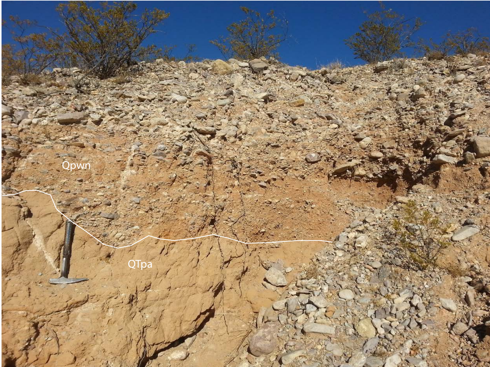
Figure 3.1. Exposure of Qpwn lying directly on QTpa with no intervening Qpwf. Photo taken circa 300815 m E, 3707700 m N.
