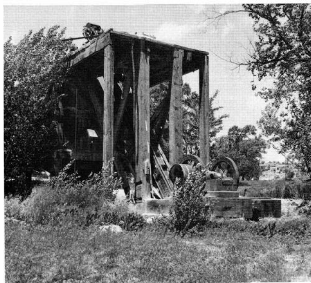
FIGURE 46—Small rock crushing unit at the Navajo No. 5 mine site, which was used to make rock dust. During the early 1920's the use of rock dust was widely adopted to help suppress coal-dust explosions. Fine limestone or gypsum was plastered on the ribs and floors, and specially constructed rock-dust barriers were filled with dry rock dust and placed overhead throughout the entries of the mine. An explosion would blow the rock dust out of these units, and the dust would confine the explosion to that particular area. This was a labor-intensive three-man rock crushing operation, which was replaced with a more efficient system designed by J. Kleiner that could be run by one man. Photo by H. B. Nickelson, 1979.
