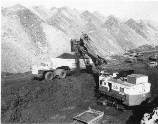
FIGURE 85—The Marion 151M shovel loading coal next to the highwall. The 120-ton, bottom-dump truck is sitting on unloaded coal next to the spoil pile. The coal bed is about 12 ft thick. Photo by Utah Construction and Mining Company, about 1965.
