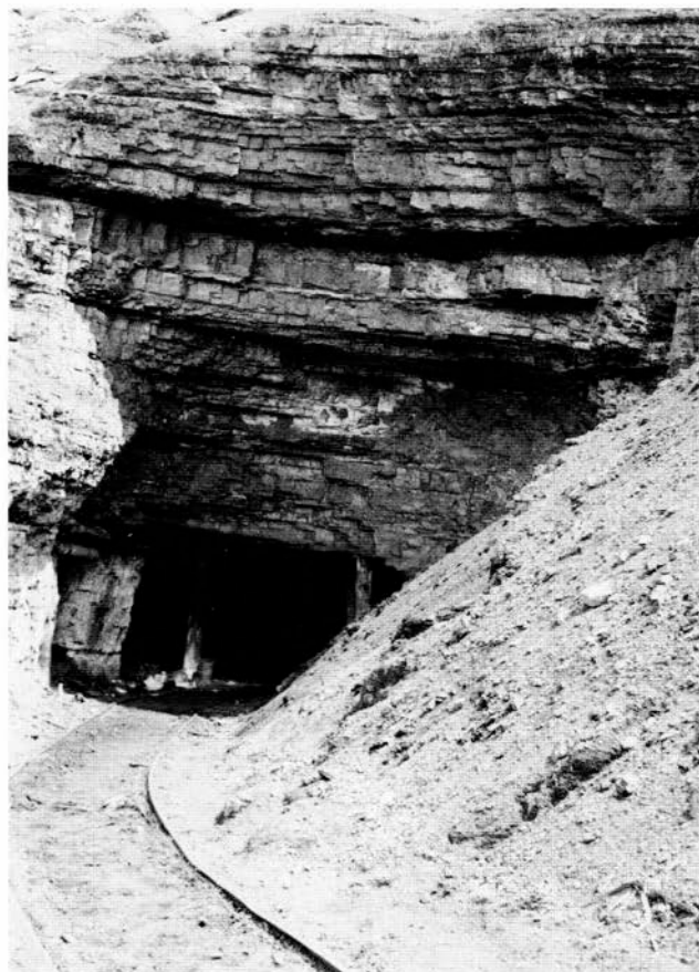
FIGURE 105—The main portal of the Prewitt No. 6 mine. The stratum exposed above the portal is the coal bed. Photo by J. J. Bourquin, April 24, 1935.
