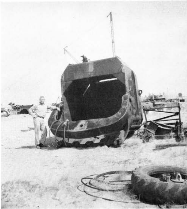
FIGURE 77—Forty to forty-five-yd 3 dragline bucket for Utah's 7900 Marion dragline, which was under construction at the time. Earl Gordon, U.S. Geological Survey, stood beside the bucket to give some idea of its size. Photo by H. B. Nickelson, spring 1961.
