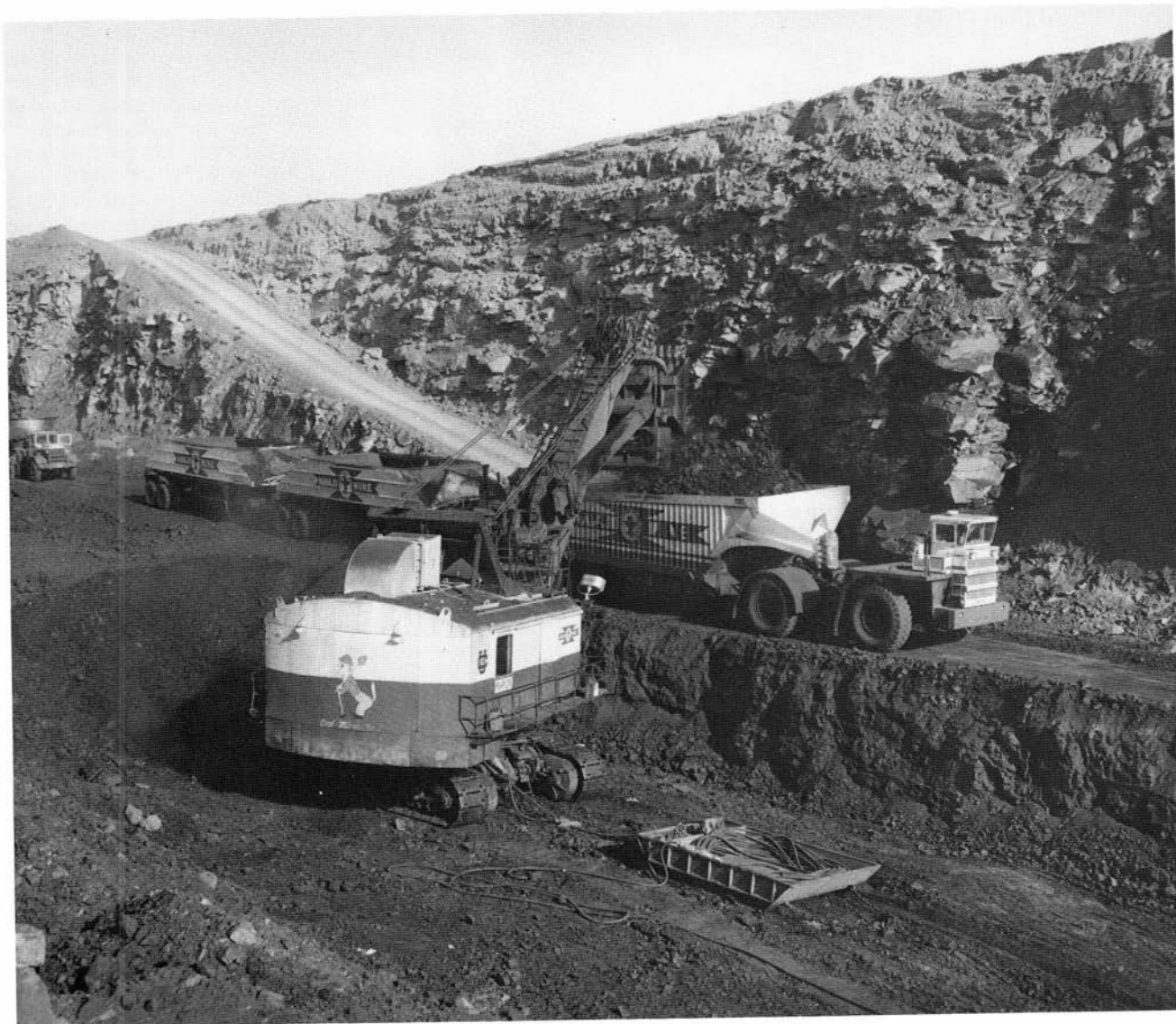
FIGURE 84—Shovel with 11-yd 3 dipper loading coal into 300-ton-capacity truck-train with 635 HP tractor and 3-tandem trailer units. A 325 HP dolly is mounted on the middle trailer for power boost. This huge prototype coal-hauling equipment proved to be unsatisfactory. Photo by Utah Construction and Mining Company, 1965 or 1966.
