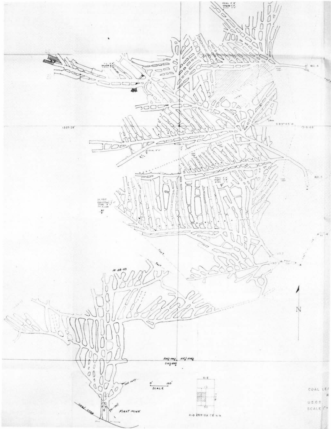
FIGURE 120—Map of the Rainbow mines showing the extent of the mine workings.
