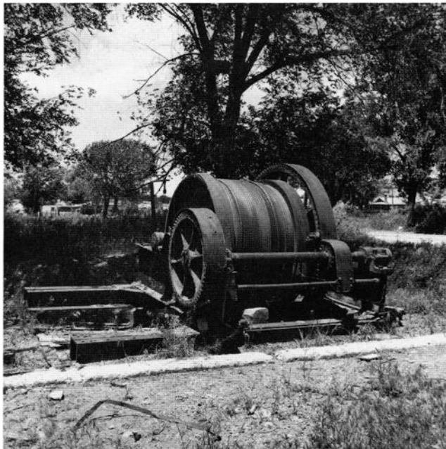
FIGURE 51—One of the underground hoists used to raise and lower the mine cars along the No. 4 NE slope in the Navajo No. 5-Gamerco mine. The hoist was removed from the mine because it caused a fire that killed seven mules. Photo by H. B. Nickelson, 1979.
