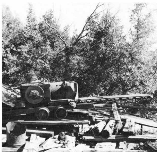
FIGURE 124—A Sullivan 11670 coal cutter. When the Rainbow-Erler No. 3 mine was abandoned, the cutter, which is on a timber truck, was removed from the underground workings and parked on the tipple. Photo by H. B. Nickelson, 1979.
