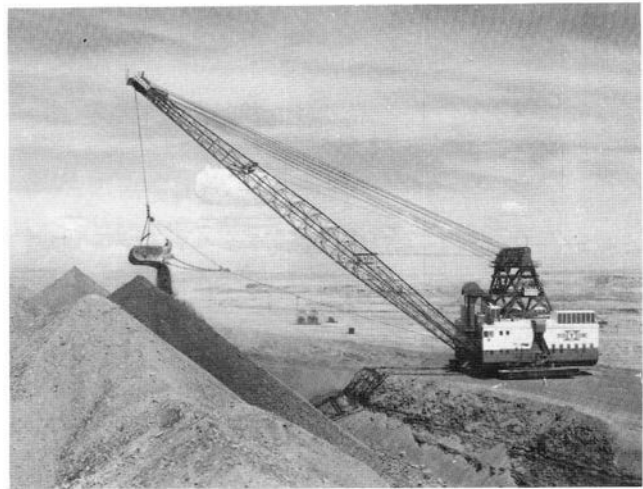
FIGURE 79—View to the north-northeast of Utah's Marion 7900 dragline in operation. Some of its specifications are as follows: 250-ft boom; 40-45-yd 3 bucket; working weight—3.9 million lbs; swing speed—1.65 rpm; walking speed—800 ft per hr; spoil radius—215-238 ft depending on boom angle; production per yr—12 million yds 3 . Photo by Utah Construction and Mining Company, about 1964.
