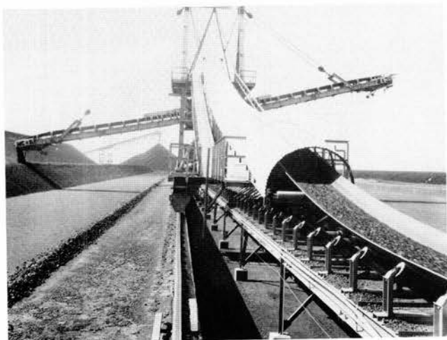
FIGURE 81—Stacker spreading crushed coal in blending piles at the Navajo mine. This machine is capable of stacking 30,000 tons of coal on each side. Photo by Utah Construction and Mining Company, about 1965.
