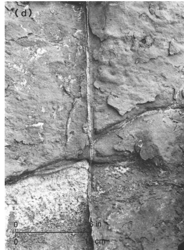
FIGURE 6.8—Morphology of individual set I fractures, Fort Lewis mine. (a) Single narrow fracture with "braided" appearance and halo of bleached rock (plan view). The morphology superficially resembles that of "deformation bands." (b) Multistrand, macroscopically segmented fracture or narrow fracture swarm with diffuse halo of bleached rock (plan view). (c) Anastomosing fractures in narrow fracture swarm (plan view). (d) Calcite-filled vein (cross-sectional view).
