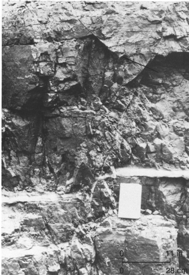
FIGURE 5.13—Small normal fault with associated fractures, Navajo mine. Width of fracture zone is indicated by a bar. Note offset tonstein. View is to west.
