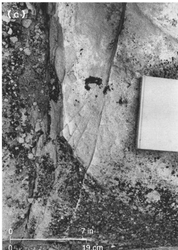
FIGURE 6.10—Fracture connectedness and termination style, Fort Lewis mine. (a) braided fracture strands. (b) Overlapping fracture strands connected by an array of thin subsidiary fractures, "ladder" structure. (c) Curved and branching fracture termination against a larger fracture. (d) Dead-end fracture termination and associated diffuse microfracture array.
