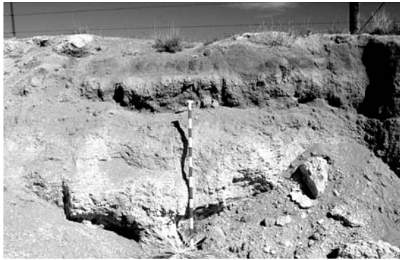
Figure 1-9. Photograph of petrocalcic soil of the Sunport surface, exhibiting Stage III+ pedogenic carbonate morphology overlain by fine- to medium-grained sand of eolian origin. The overlying eolian sand commonly forms an extensive cover over the carbonate of the Sunport surface. Scale is 1.5 m.
