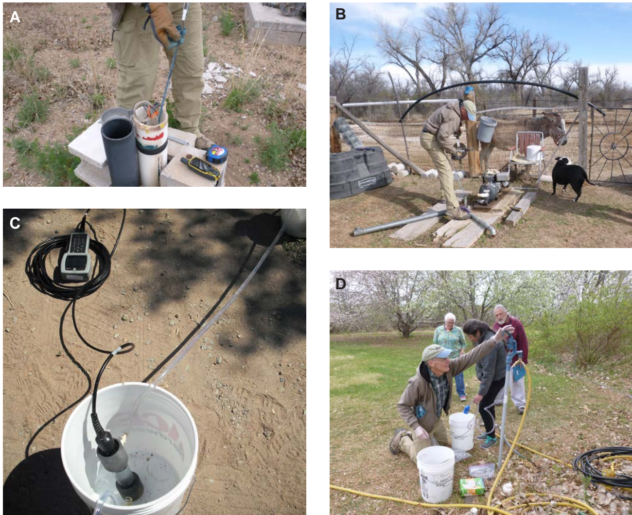
Figure 5. Images of (a) water level measurement taken to measurement point, (b) raising the steel tape, (c) measuring water quality field parameters to ensure a characteristic groundwater sample, and (d) taking a filtered groundwater quality sample.
