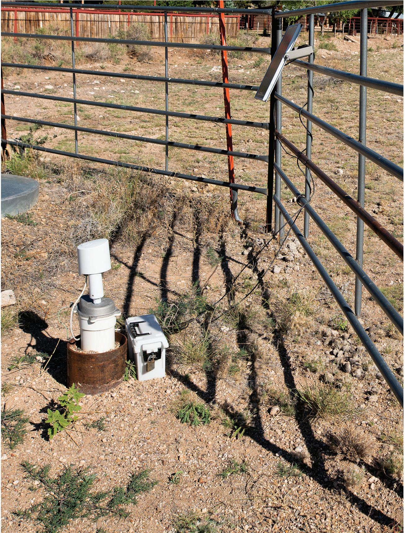
Groundwater levels can be monitored using acoustic devices with telemetry, as shown here.
