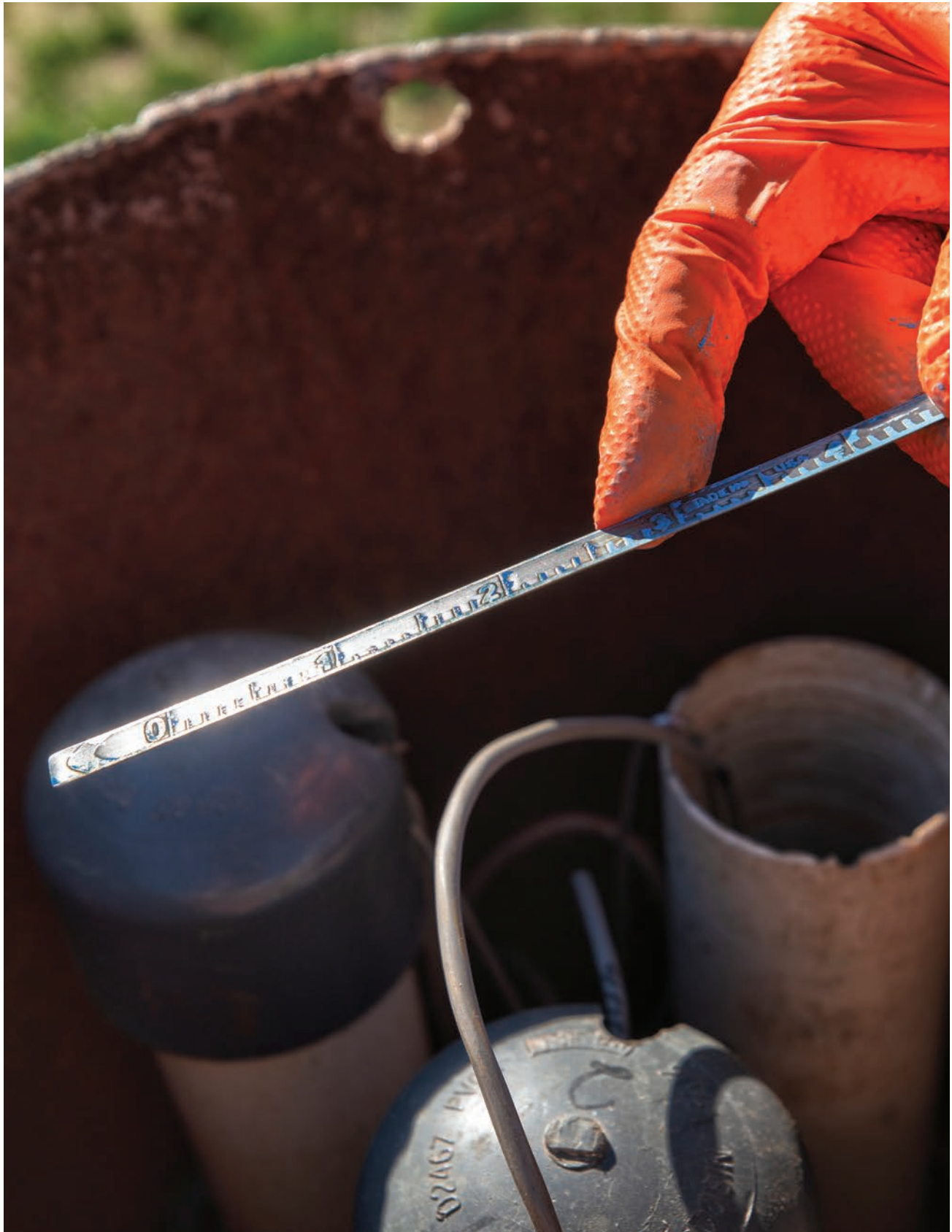
Steel tapes with graduated markings are the preferred and most accurate method for measuring depth to groundwater. Photo by Christi Bode, Moxiecran Media LLC
