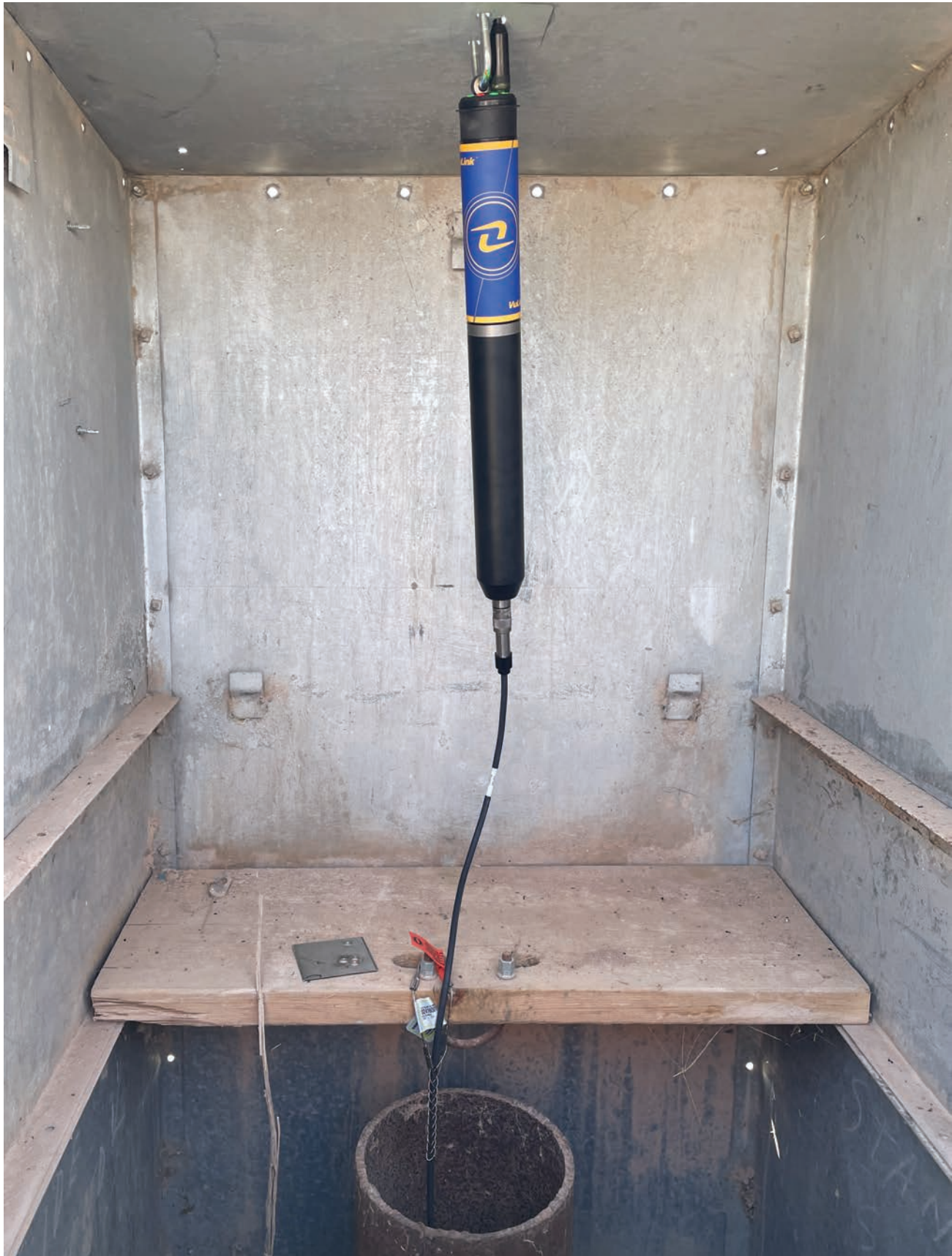
Depth to water measured in real time using a pressure transducer with telemetry.
