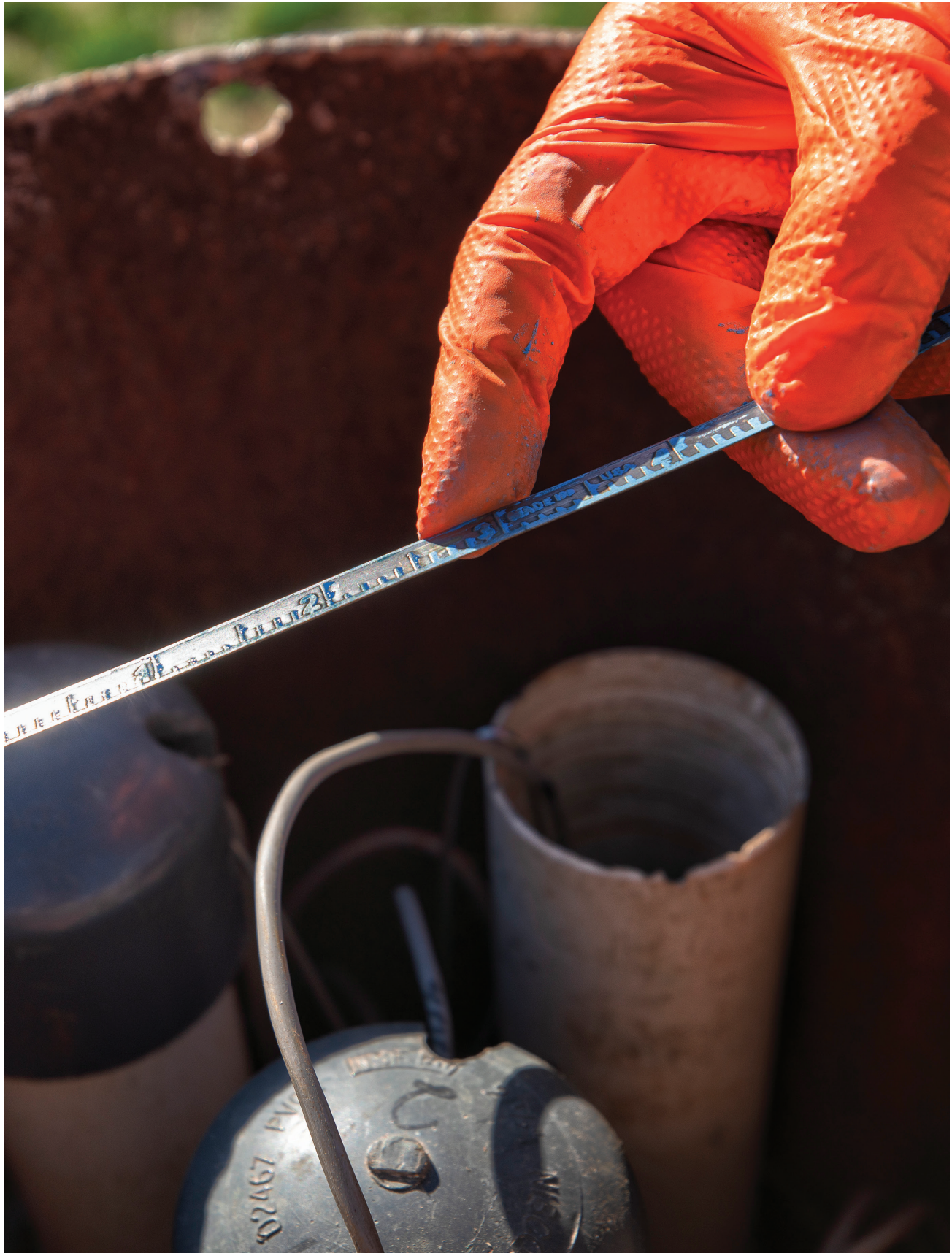
Water mark on a steel water-level measuring tape. Photo by Christi Bode, Moxiecran Media LLC
