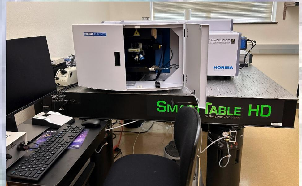
New state-of-the-art Horiba LabRAM HR Evolution confocal Raman microscope equipped for solid, gas and liquid experiments.
