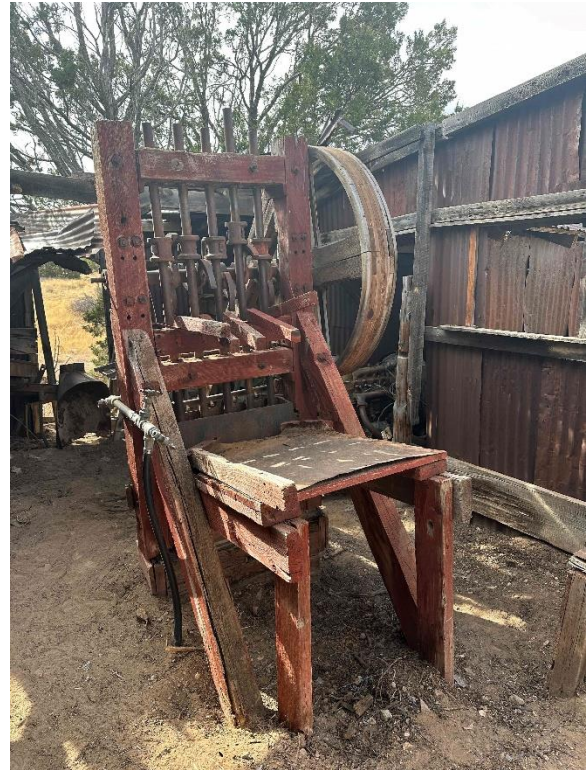
Golden Stamp mill (built c 1885) behind the Henderson Store, Golden, NM. Donated by Desiri and Al Pielhau.
