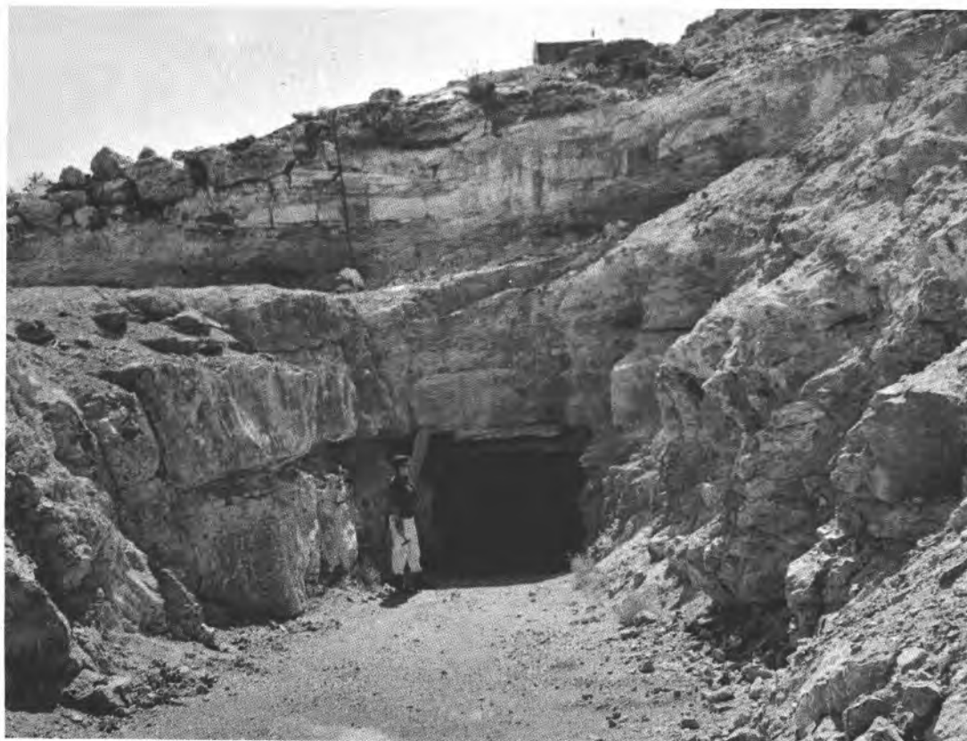
Portal of an Exploration Adit at a Lead-Barite-Fluorite Prospect
