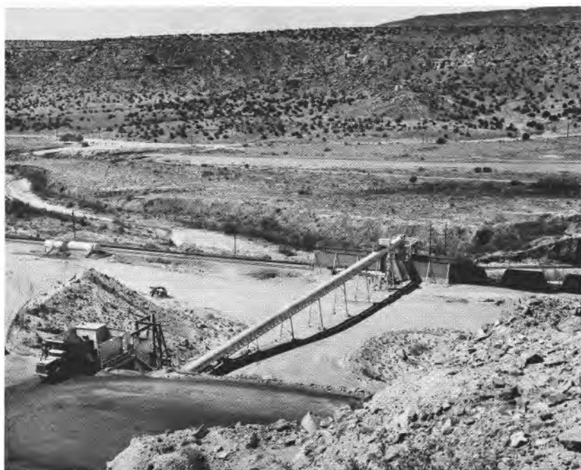
Uranium ore being loaded into new air-dump hopper cars at Jackpile mine. (Courtesy of Santa Fe Railway)
