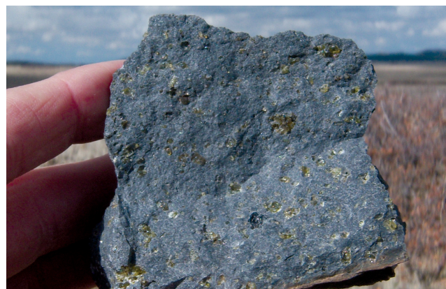
FIGURE 28. The photograph shows the phenocryst texture of olivine-rich basalt ( Qolpb ; 2.41 Ma); virtually every phenocryst is olivine although there are a few black-augite and white-plagioclase phenocrysts. Many of the "true" basalts (see Appendix 2) have extremely abundant phenocrysts of olivine \pm augite \pm plagioclase.
